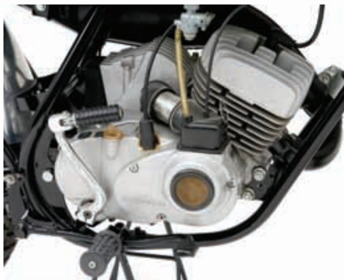
The green-meanie Centurion came out of the box just like this — no lights, no excuses. Below: The disc-valve system — and the lack of a carburetor — give the G31M two-stroke a decidedly unique look.
